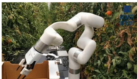
Fig 1. Harvesting robot for tomatoes
